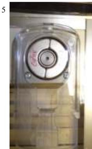
**✓** In this picture the base plate is positioned so that the internal magnet is clearly visible within the 'keyhole' shape of the base plate. This correct alignment will allow the external and internal magnets make a firm connection through the glass. Even slight overlapping of the internal magnet will prevent the coupling between the two magnets. Ensure that the base plate is straight and parallel to the frame.
