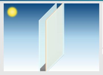
Pane 1 PLANICLEAR (4 mm) Cavity 1 ARGON (90%) / AIR (10%) / 16 mm PLANITHERM ONE II Pane 2 PLANICLEAR (4 mm)
