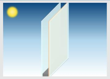
Pane 1 PLANICLEAR (4 mm) Cavity 1 ARGON (90%) / AIR (10%) / 16 mm PLANITHERM TOTAL+ FG Pane 2 PLANICLEAR (4 mm)
