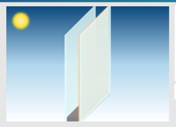
Pane 1 PLANICLEAR (4 mm) Cavity 1 ARGON (90%) / AIR (10%) / 20 mm PLANITHERM TOTAL+ FG Pane 2 PLANICLEAR (4 mm)
